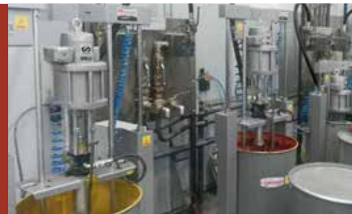
PM35 60:1 ratio Dynamic-Primer lubrication equipment pump package for dispensing heavy greases.
